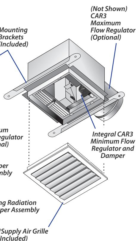
\*ZRT-S-F model supplied with Supply Grille (shown). ZRT-F model supplied with Exhaust/Return Grille (not shown).
