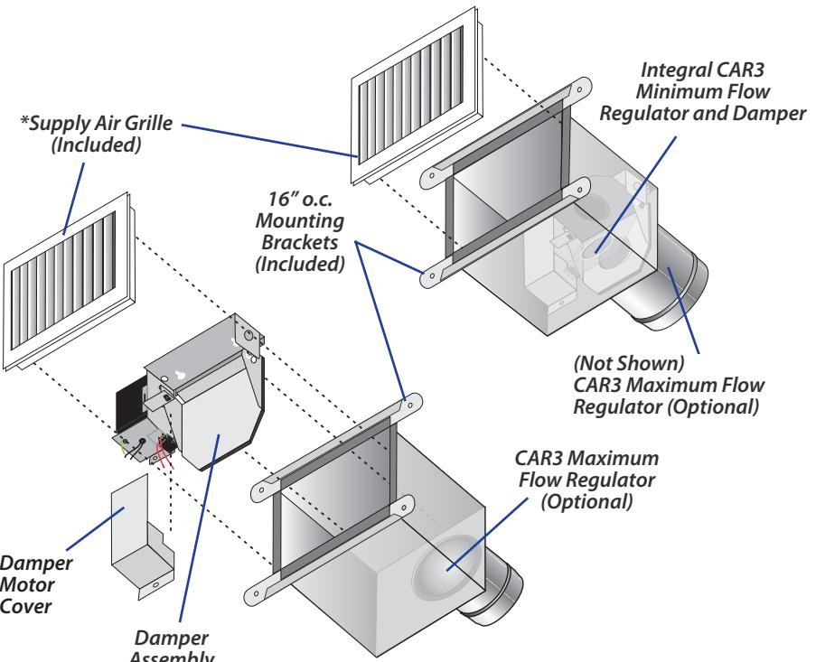
\*ZRT-WS model supplied with Supply Grille (shown). ZRT-W model supplied with Exhaust/Return Grille (not shown).
